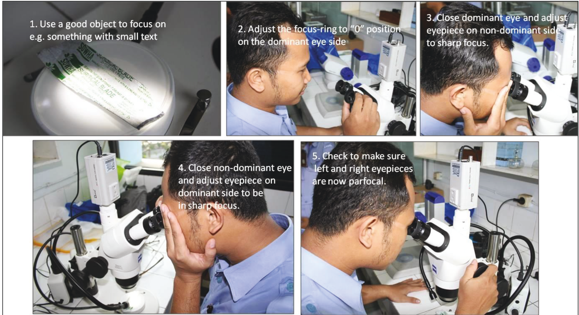
Figure 37. Steps in the set-up of microscope to ensure eyepieces are parfocal, prior to commencing otolith readings. Note: The ergonomics of the work set-up shown are not ideal. The microscope is too low (or person is sitting too high) and the user has to 'hunch' over to see down the eyepieces.
