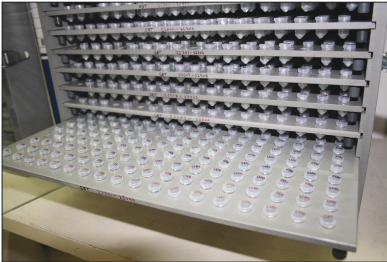
Figure 22. The cabinets shown are used by CSIRO in Hobart for storing tuna otoliths. Each cabinet, of dimensions 40cm x 40cm x 40 cm, has capacity for 13 shelves of otolith sample vials, with approximately 306 vials per shelf if the holes in the shelves are in straight columns. This provides a total storage capacity of 3,978 vials per cabinet.
