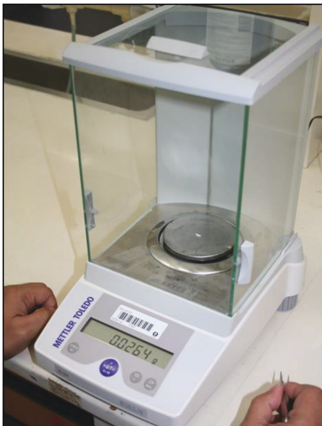
Figure 24. Obtaining an accurate weight for your otoliths, prior to embedding, is important. Handle the otoliths with great care, using fine forceps, and always over the lab bench and not over the floor!
