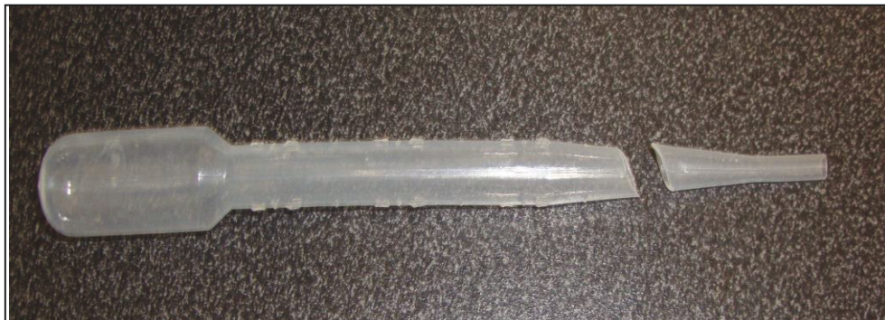
Figure 36. Plastic pipette with tip cut off. Note the angle of the cut.
