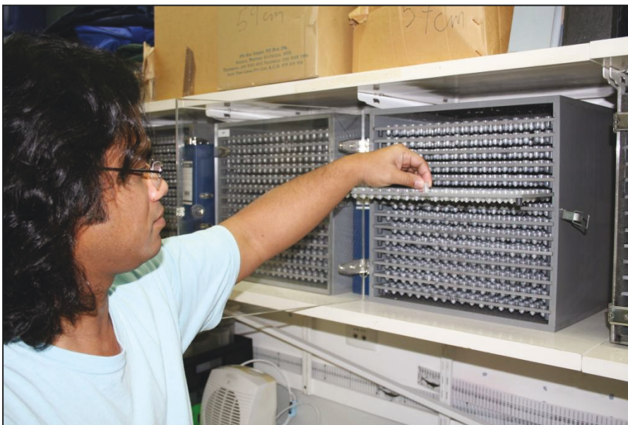
Figure 21. Small vials and custom-made cabinets provide a relatively space efficient method of storing a large number of otoliths. Such a storage system is only suitable for small to medium-size otoliths.
