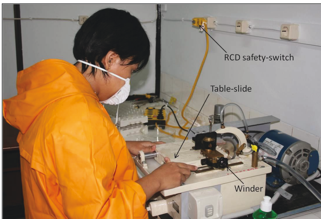
Figure 32. Sectioning otoliths on the GemMasta GS6D.
