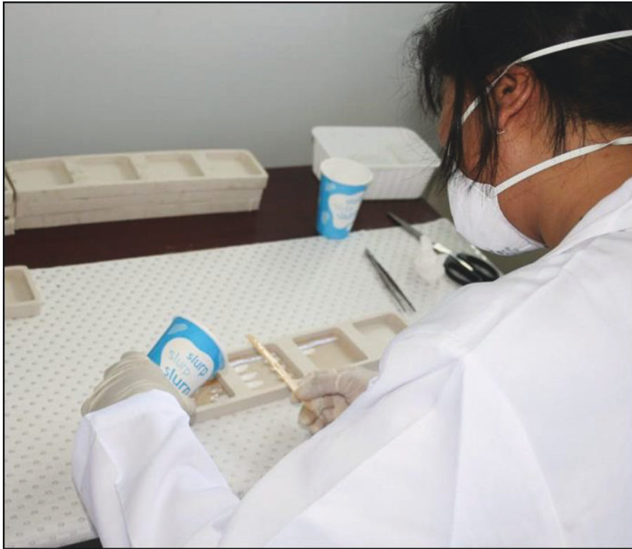
Figure 27. Pouring resin over otoliths that have already been organised in the compartments of the mould, and using a stick to wipe excess resin from the lip of the cup to prevent messy drips.
