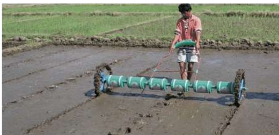
Figure 8.31. A 6 drum (12 row) 2.4 m wide drum seeder ( www.knowledgebank.irri.org ).
