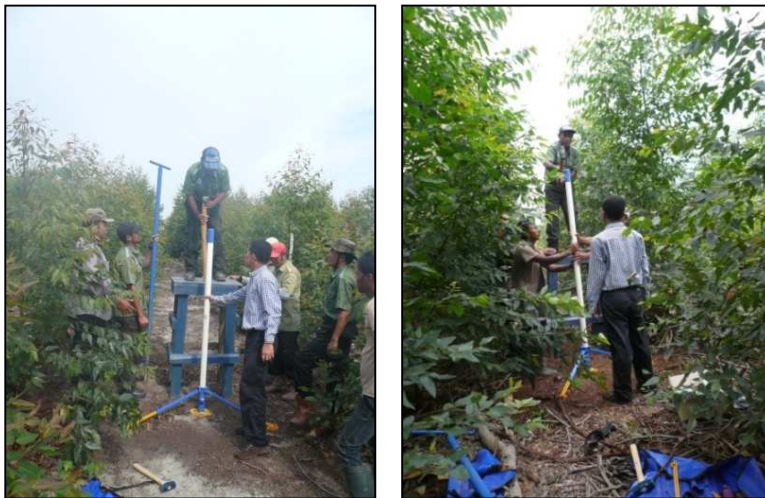
Figure 2 – Installation of soil moisture probes at Teso East, March 2012 (a) Eucalypt , (b) A. mangium .
