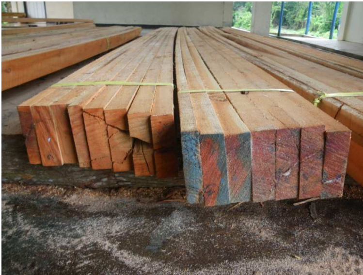
Figure 50: A comparison of end-splitting between a log that had been wax-sealed and one that had not.
