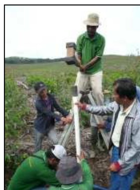
Figure 3 (a) Lipat Kain site, November 2012, (b) installation of soil moisture access tube in plot T6R1.
