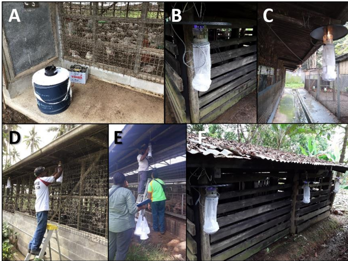
Figure 5. Different mosquito traps types employed for this project: BG Sentinel trap (A), CDC light trap with incandescent light (B) and UV light (C). Traps being hung and changed at EBC farm (D), Boroma Piggery (E) and Kiunga (F).
