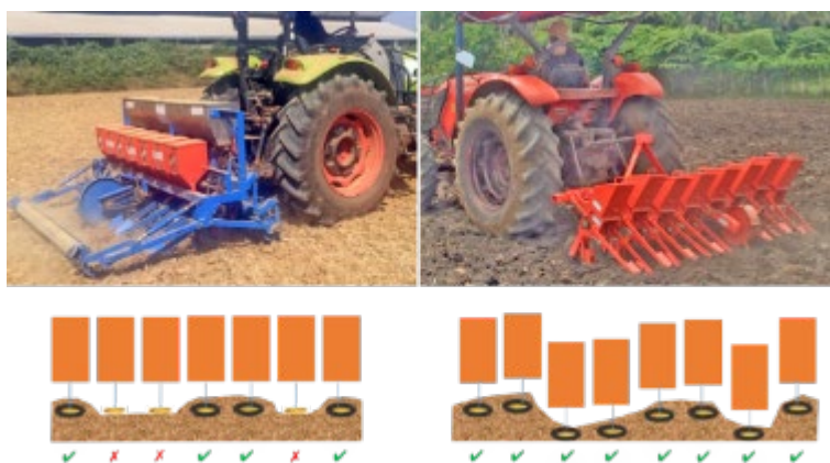
Figure 77. Comparison of Kid and Kubota planters for ground engagement and seed placement
