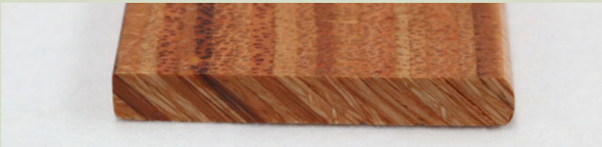
Figure 10.17. Multilaminar wood section sawn across the end grain at 45^\circ to the veneer direction.
