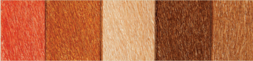
Figure 10.14. VJ style wall panelling using medium-density cocoveneer on medium-density fibre boards (MDF). Surface finishes included red (left), golden, clear (middle), dark brown and light brown (right) stains.
