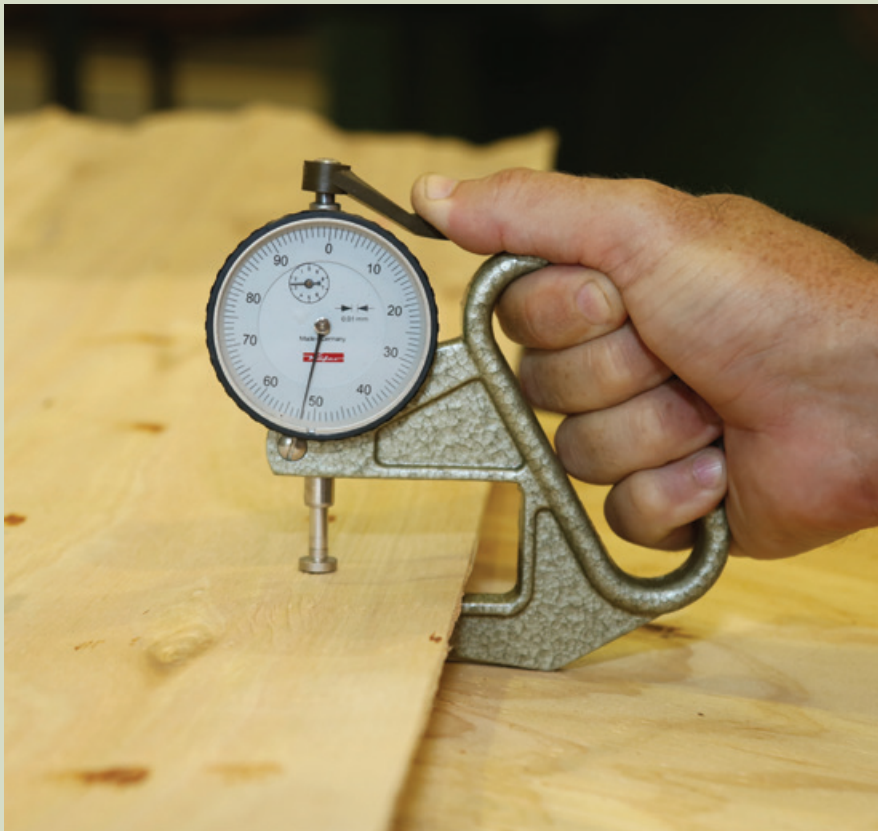
Figure 8.4. A hand-held dial gauge used to measure veneer thickness.
