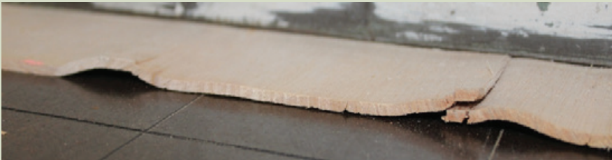
Figure 7.5. Waviness can cause an overlapping when pressed flat
