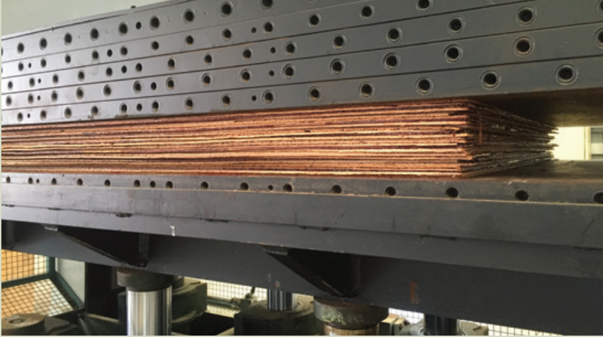
Figure 10.6. Cocoveeners being pressed into a panel product.
