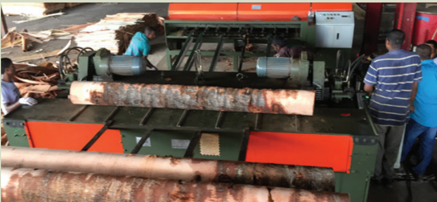
Figure 10.4. Spindleless peeling trial in the commercial ply mill at Labasa, Vanua Levu, Fiji.
