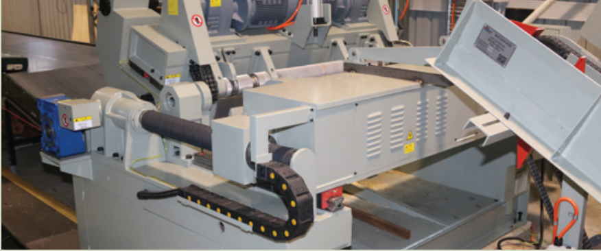
Figure 5.4. An example of a spindleless lathe.
