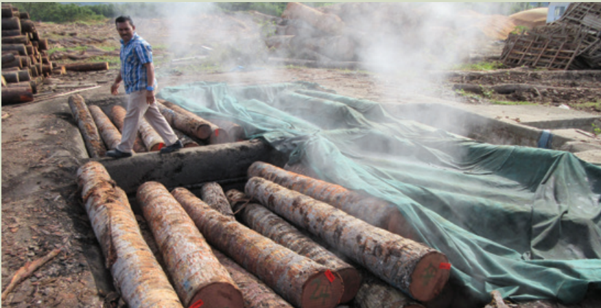
Figure 4.6. Coconut peeler billet pre-conditioning using a steam chamber.
