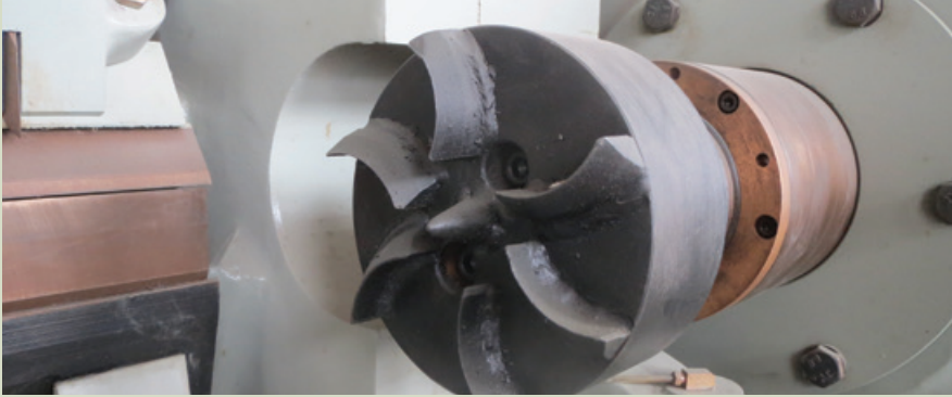
Figure 5.3. 'Chucks' or spindles on a spindled lathe.
