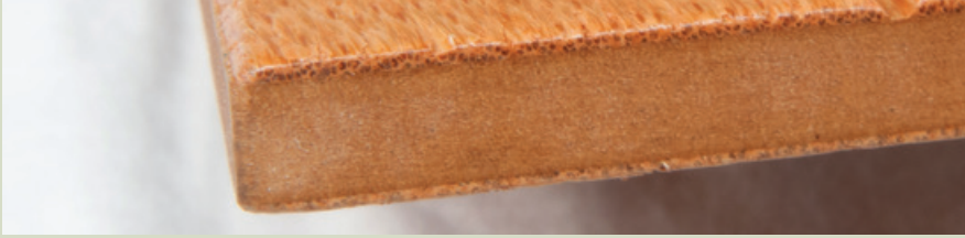
Figure 10.13. Veneer overlay panel using medium-density cocoveneer on medium-density fibre boards (MDF).
