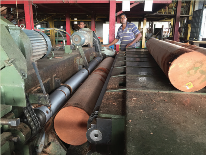
Figure 4.7. Cylindrical coconut logs after round-up and ready for peeling.
