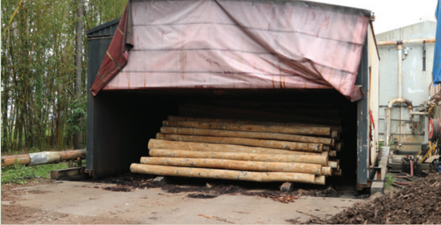
Figure 4.5. Log pre-conditioning using saturated steam.
