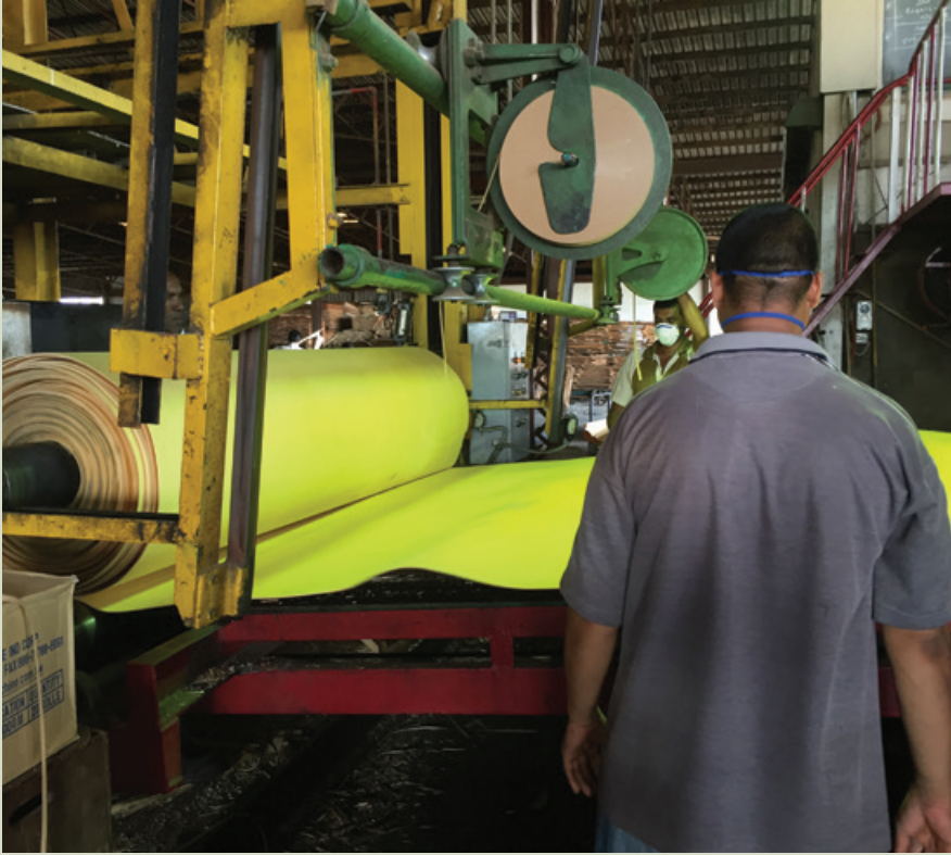
Figure 6.2. Veneer being coiled in preparation for a separate clipping operation.
