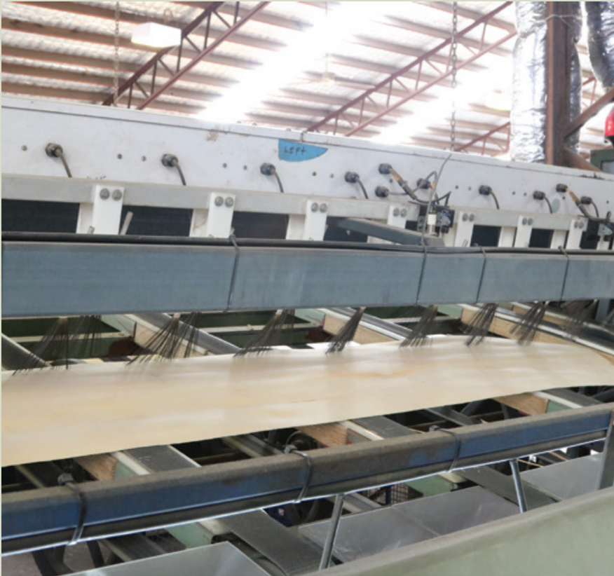
Figure 8.9. In-line veneer moisture measurement.
