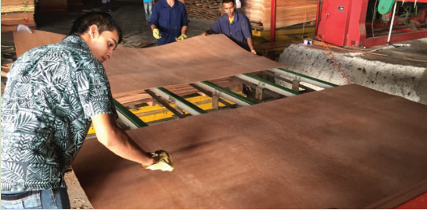
Figure 6.3. Coconut veneer clipped and ready for drying.
