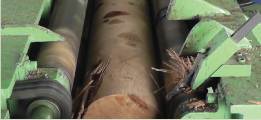
Figure 10.3. Spindleless peeling trial in the experimental facility at Nasinu, Viti Levu, Fiji.
