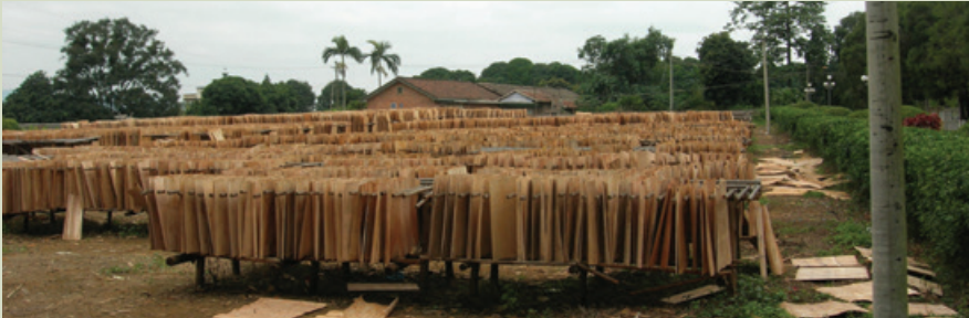
Figure 6.4. Air-drying hardwood veneer sheets in Vietnam.
