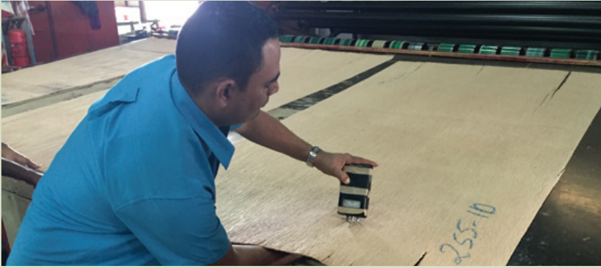
Figure 8.7. A hand-held resistance moisture meter.
