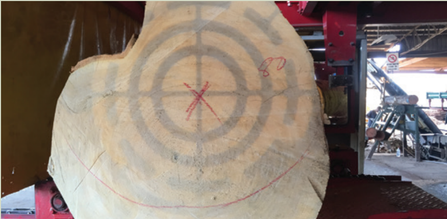
Figure 4.8. Visual aids such as a light stencil can assist the lathe operator in positioning the lathe spindles.
