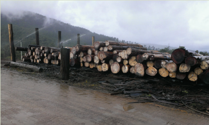
Figure 4.2. Using water sprays in a log storage yard prevents excessive or rapid drying and deters insect and fungal attack.
