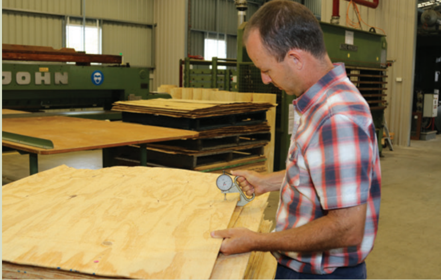
Figure 8.5. Routine checking for veneer thickness variation.
