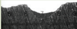
Figure 10.1. Chipped knife edge caused by a high-density vascular bundle during peeling at ambient temperature.
