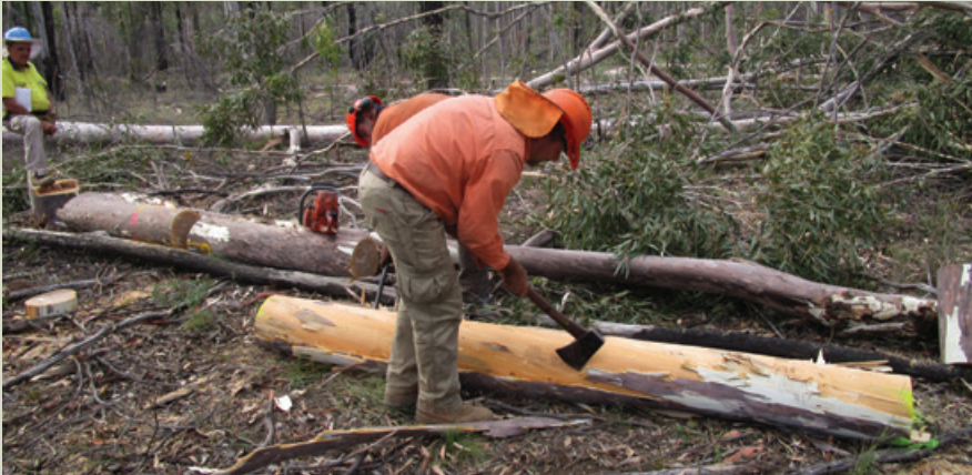
Figure 4.3. Removing bark from a hardwood log with the cutting face of an axe.
