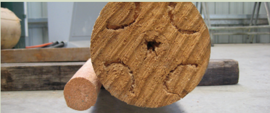
Figure 5.5. A 45 mm coconut peeler core (left) produced from a spindleless veneer lathe, compared with a 130 mm softwood peeler core produced from a standard, commercial spindled lathe.
