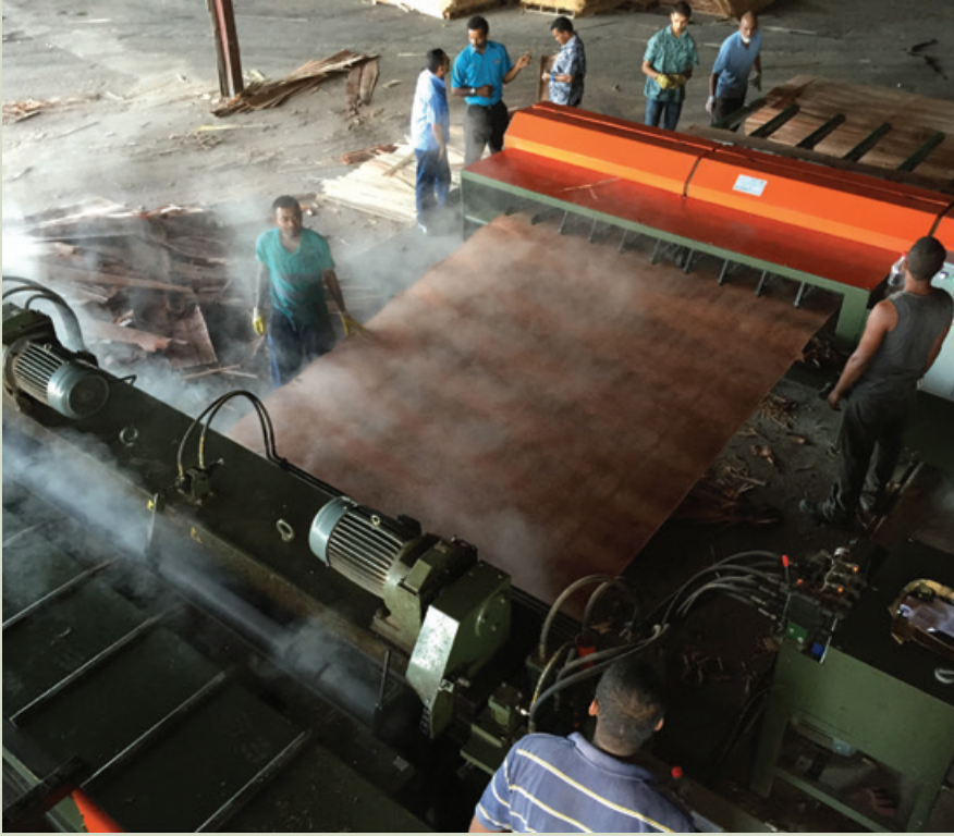
Figure 5.6. A coconut log being peeled with a spindleless lathe.
