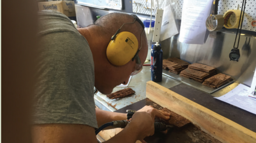
Figure 10.8. Bond testing using the chisel test.
