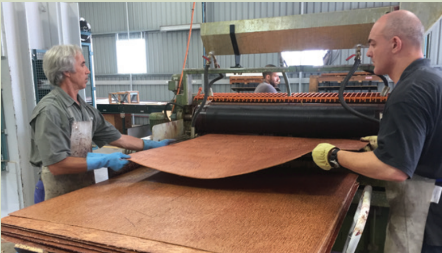
Figure 10.5. Coconut palm veneers being passed through the glue spreader in preparation for plywood manufacture.
