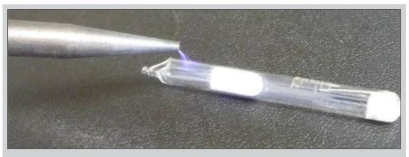
Figure 4.6 Checking for a vacuum with a high-frequency spark tester
