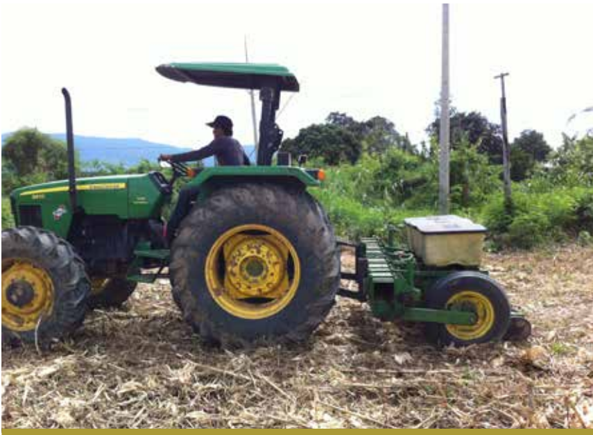
Figure 10. No-till planting into 5 t/ha maize residue using a 3-row John Deere Maxemerge planter. Photo: R. Martin
