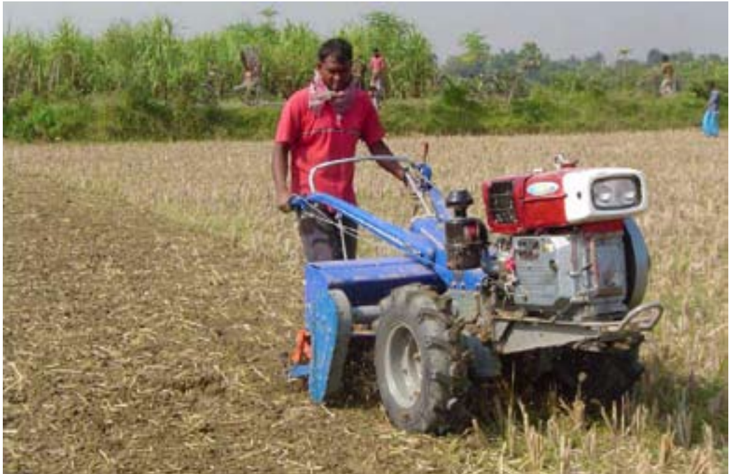
Figure 6. Tilling and line sowing in one pass using a power-tiller-operated seeder (PTOS) (Photo: E.M. Haque, CIMMYT Bangladesh)
