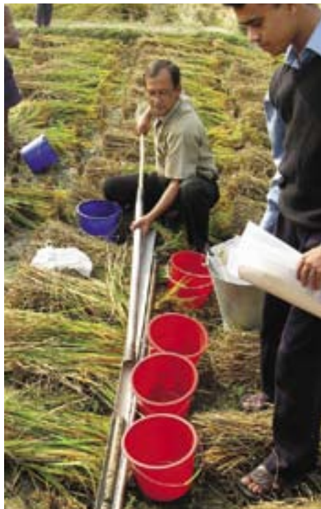
Figure A1. Soil coring: (a) driving the steel coring tube into the ground with the wooden hammer; (b) extracting the core tube using the jack; and (c) placing the extracted core into the cutting tray for cutting into depth layers and bagging
