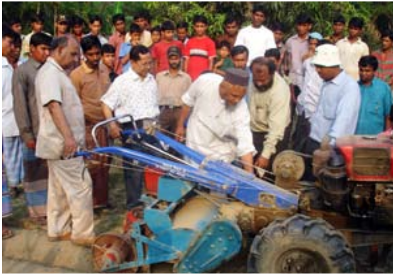
Figure 2. New bed former-planter attached to a power tiller being demonstrated. Bed compaction is sufficient to support the weight of a person on the ridge. This is a single-pass operation from untilled to seeding (Photo: E.M. Haque)
