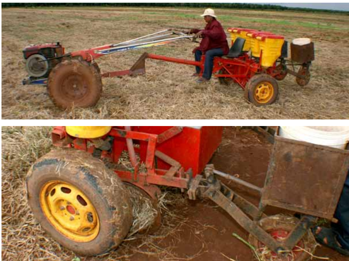
FIGURE 22. No-till disc planter sowing soybean into brachiaria grass mulch, Kampong Cham province (top) and close-up of disc tyne and press wheel (bottom)
