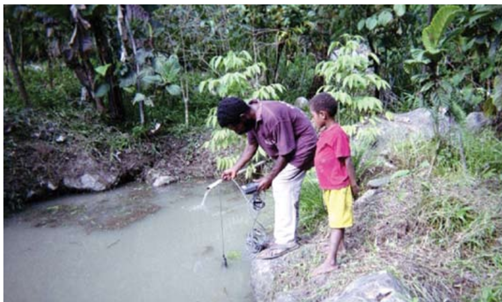
Technical officer Mr Kaupa Kia measuring pH in a fish pond in Simbu province
