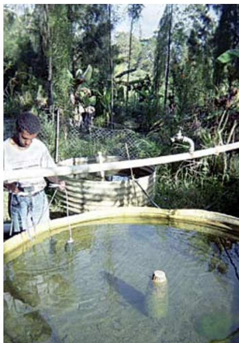
Technical officer Mr Micah Aranka taking DO (dissolved oxygen) readings at Mr Peter Gundil's carp hatchery in Simbu province
