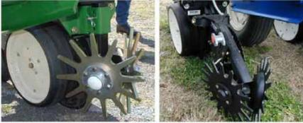
Finger wheel attached to opener frame
