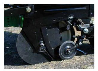
Figure 202 shows a gravity drop seed delivery system using a long, rigid, dropper tube with a rearward deflection to convey seed from a precision meter to a single disc type furrow opener.
