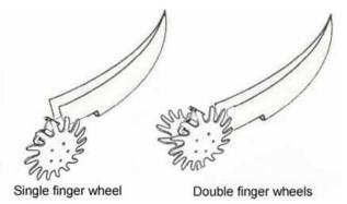
Figure 121: Single and double finger wheel covering devices
