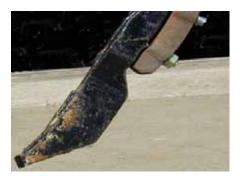
Figure 87: A typical knife type tine opener
