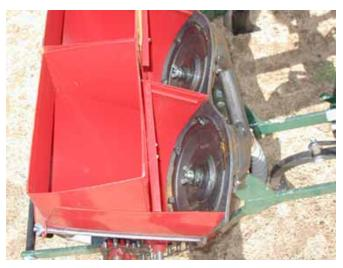
Figure 181: Twin inclined plate meters delivering seed to a common delivery tube
