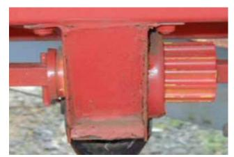
Figure 169 shows the front view of a fluted roller type of external force feed seed meter with the fluted roller moved axially so as to have no exposure to the seed.
