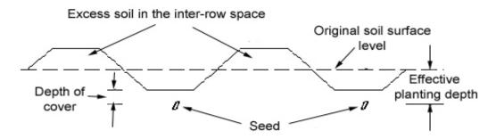
*Figure 3: Alteration of soil surface profile to facilitate planting deeper to moisture*
