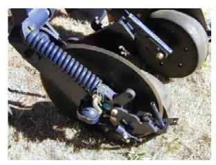
Figure 161: A dedicated gauge wheel type of the trailing arm system of depth control
