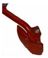
Figure 94: Rearward curved shoe type opener and seed placement device
