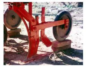
*Figure 160: A furrow opener utilising a rear gauge wheel type of the trailing arm system of depth control*
