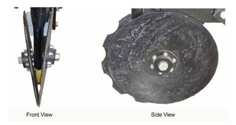
Figure 76: A staggered twin inclined double disc coulter with a notched leading coulter
