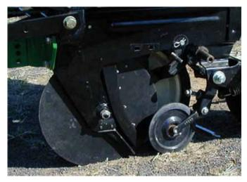
Figure 69: A typical seed placement device for use with single disc coulter type openers
