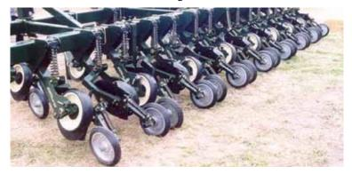
Figure 66: Openers arranged in opposed pairs across the full width of the machine
