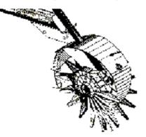
Figure 100: A punch type furrow opener for planting through residue
