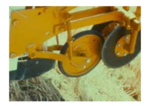
Figure 111: Double disc coulter type covering devices following a seed-firming wheel
