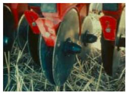
Figure 80: A rear view of a dedicated triple disc coulter type furrow opener
