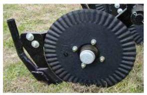
Figure 21: A ripple disc coulter type soil and residue cutting device
