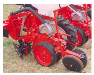
Figure 155: A planter utilising a 'dedicated gauge wheel' type of depth control
