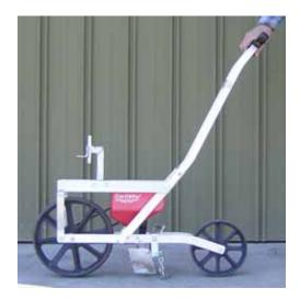
Figure 12: A single-row, hand-pushed, human-powered, precision planter
