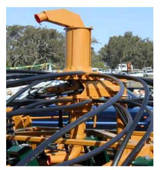
Figure 211: Seed and fertiliser heads incorporating hydraulically driven components
