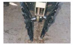
Figure 132: The typical shape of finger wheels used as a row specific seedbed firming device
