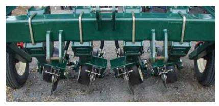
hand side of the machine opening in one direction and all the openers on the right hand side of the machine opening in the opposite direction as shown on the 4-row planter in Figure 65.
