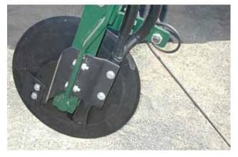
Figure 120: A single finger type covering device
