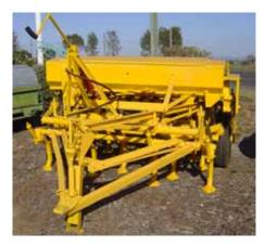
*Figure 11: A 14-row, trailed, tractor-powered drill planter*
