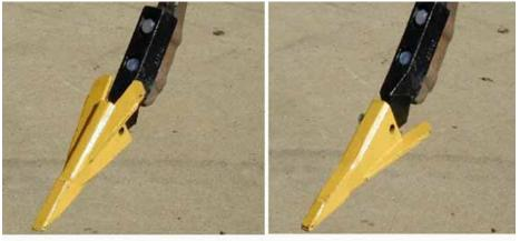
Reversible point with wings up Reversible point with wings down Figure 85: An example of a reversible point type opener
