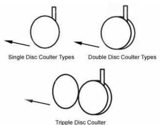
Figure 56: General types of disc coulter furrow openers
