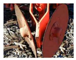
Figure 35: An example of an aligned, plain double concave disc coulter type concave disc coulter
