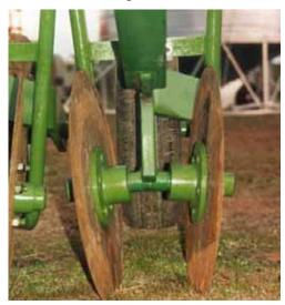
Figure 67: Opposed single compound angle disc coulters mounted on a common arm
