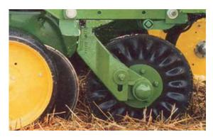
Figure 20: A bubble disc coulter type soil and residue cutting device
