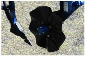
Figure 22: A wavee disc coulter type soil and residue cutting device
