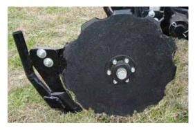
Figure 19: A notched disc coulter soil and residue cutting device
