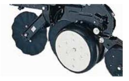
Figure 23: A fluted disc type soil and residue cutting device
