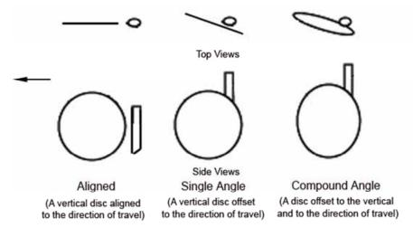
Figure 57: Types of single disc coulter furrow openers
