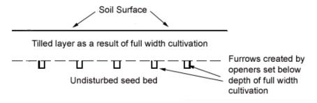
Figure 2: The concept of separating tillage and seeding functions
