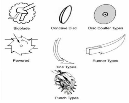
*Figure 46: Common types of furrow opening devices*
