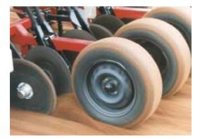
The particular design shown in Figure 68 has been developed for twin row planting in frictional soils. Both discs share a common press/depth wheel, the operation of which is shown in Figure 67.
