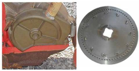
Side view of a vacuum disc seed meter
