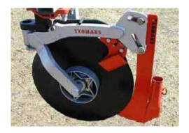
*Figure 18: A plain disc coulter type soil and residue cutting device*
