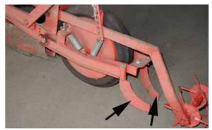
Figure 114: Opposed knife type covering devices
