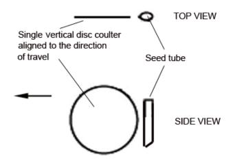
Figure 58: Single, aligned disc coulter opener type
