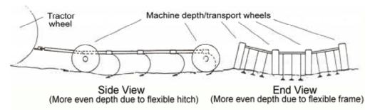
*Figure 148: A trailed, flexible hitch, 4 bar, 3 section flexible-framed planter operating on an irregular surface*
