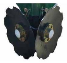
Figure 36: An example of a staggered, notched double
