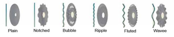
Figure 17: Typical cutting edge profiles for each general disc coulter type
