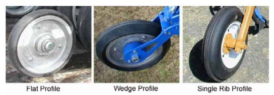
Figure 126: Some types of over-centre press wheel profiles
