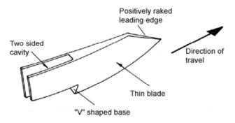
Figure 50: Stub runner type opener
