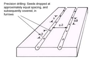
Figure 6: The 'precision drill' planting pattern
