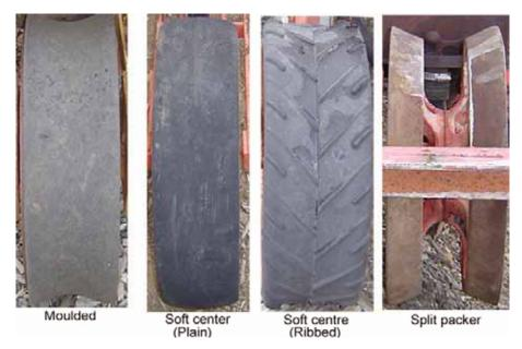
Figure 128: Zero pressure press wheel types
