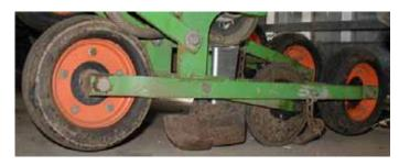
Figure 103: A seed-firming wheel following a runner type furrow opener
