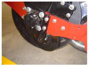
Figure 70: A rotary disc type seed placement device on a single-angle disc coulter opener
