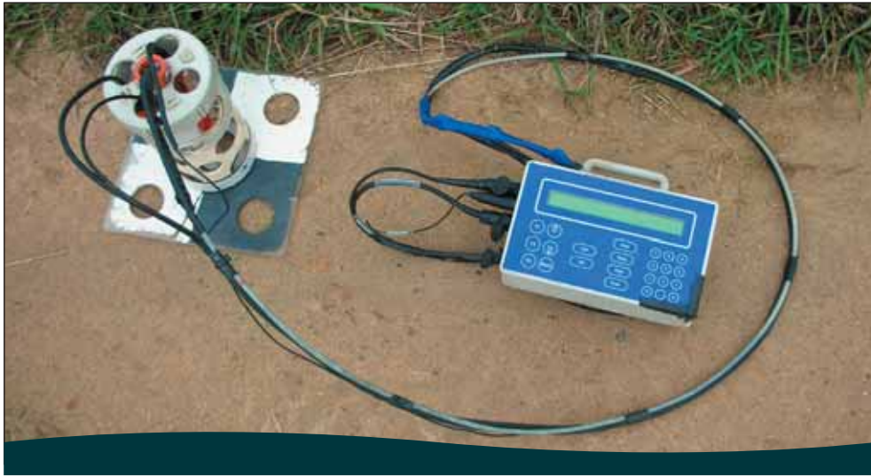
Figure 3.5 A hand held water quality data logger and probe system, with secchi attached below the probe.
