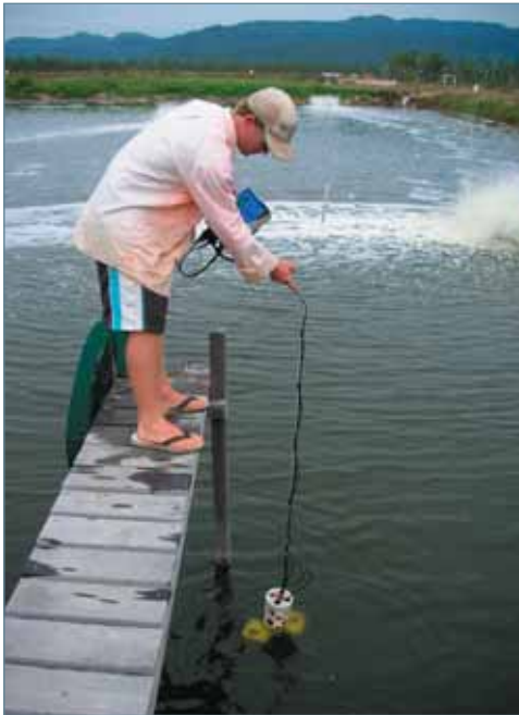
Figure 3.7 (right) A secchi attached to a water quality monitoring probe for daily pond monitoring
