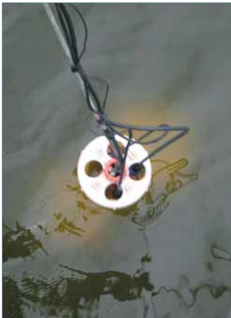
Figure 3.9 (right) The secchi in the water column at the transition depth. This is the depth for the secchi reading
