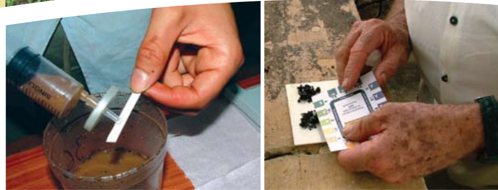
Figure 7. Rapid tests are available for determining available soil nitrate (left) and pH (right).
