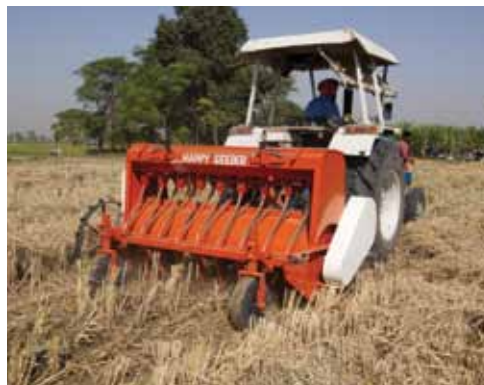
Replace the plough with specialised zero-till seeders.
