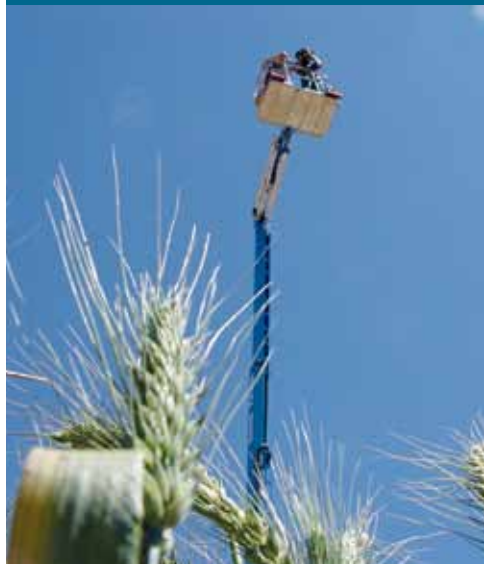
David Deery manning the 15-metre High Resolution Plant Phenomics Centre imaging tower used to take infrared thermography images of wheat crops. The imaging technology is being used to improve the water productivity of wheat in dryland farming systems.
