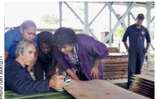
Measuring the thickness of the cocoveneer—Eric Littee of the Queensland Department of Agriculture and Fisheries with team members from Fiji's Department of Forestry.
