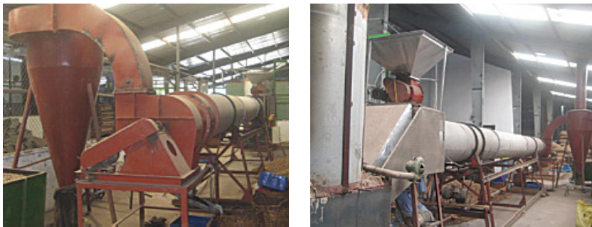
Figure 5. Equipment for heat-moisture treatment of raw cashew (capacity 1 t/hour) using steam-drying technology designed by Sub-Institute of Agricultural Engineering and Post-Harvest Technology (shown from either end of the machinery)
