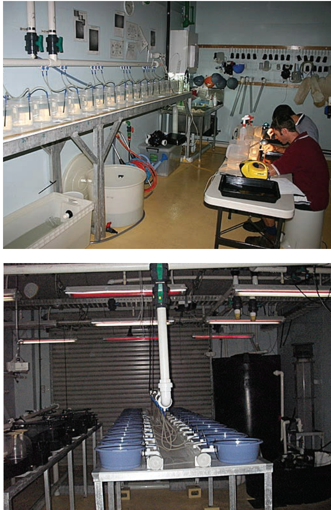
Figure 2. Photos of larval rearing systems using 3L water jugs and 5L tubs for small-scale, replicated experiments
