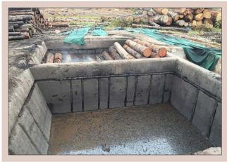
**Figure 3.21.** Log pre-conditioning using hot water soaking.
