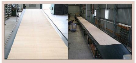
Figure 7.2. Examples of straight tracking.
