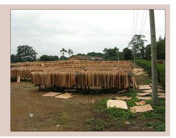
**Figure 5.4.** Air-drying veneer sheets in Vietnam.
