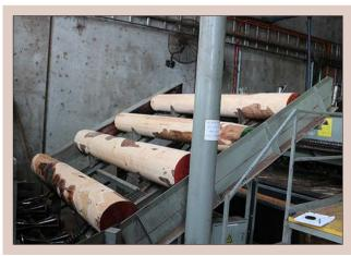
**Figure 3.24.** Cylindrical logs after round-up, and ready for peeling.
