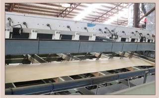
**Figure 7.12.** In-line veneer moisture measurement.
