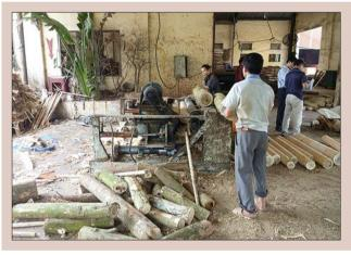
Figure 3.23. Combining debarking and log round-up in one operation in Vietnam.
