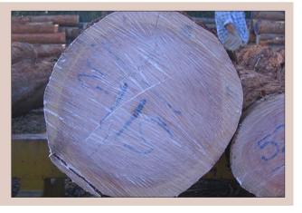
Figure 3.15. Log ends coated with a wax-based end-sealer.
