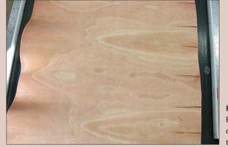
**Figure 7.6.** Buckling and splitting on opposite edges of the veneer ribbon.
