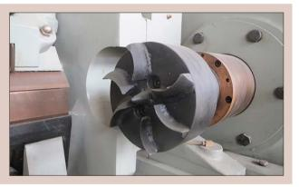
**Figure 4.3.** 'Chucks' or 'spindles' on a spindled lathe.
