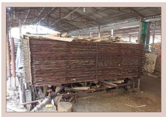
**Figure 12.7.** Veneer press drying.
