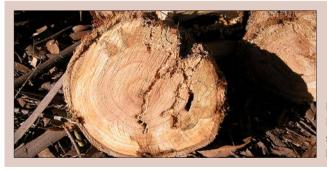
**Figure 3.9.** Holes of varying sizes due to insect borer damage.
