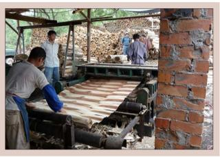
Figure 5.2. Veneer ribbon being coiled in preparation for a separate clipping operation.
