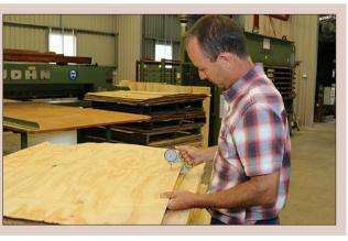
**Figure 7.8.** Routine checking for veneer thickness variation.
