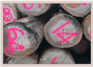
**Figure 3.17.** S-hooks on log ends can minimise end-splitting.
