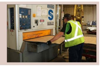
**Figure 9.9.** Sanding veneers to reduce thickness variation.
