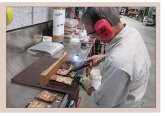
**Figure 10.1.** A pneumatic chisel is used to separate veneers in the chisel test method.
