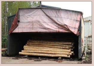
Figure 3.22. Log pre-conditioning using saturated steam.
