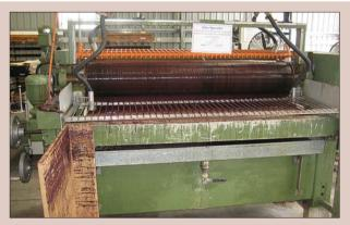
**Figure 9.1.** A double-roll glue spreader.
