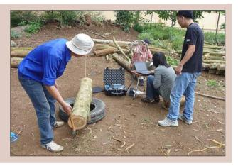
**Figure 12.3.** Log stiffness assessment using the Bing acoustic method.
