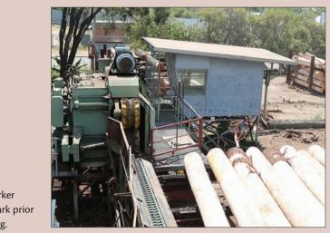
**Figure 3.20.** A ring debarker removing bark prior to processing.
