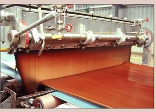
**Figure 9.3.** A curtain coater. Source: Wesbeam Pty Ltd, Australia.
