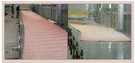
Figure 7.3. Examples of mis-tracking.
