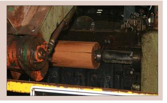
**Figure 4.4.** End-splitting during peeling with a spindled lathe.
