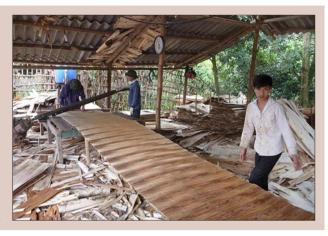
**Figure 5.1.** Veneer sheets being clipped manually by guillotine in Vietnam.
