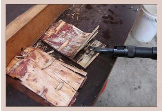
**Figure 10.2.** Veneers are separated to assess wood fibre failure.
