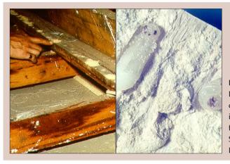
Figure 11.2. Lyctid beetle damage to wood including larvae and frass. Photos: Ted Stubbersfield (left); Doug Howick (right).
