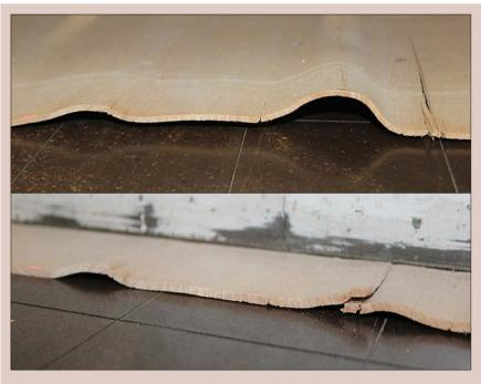
Figure 6.14. Waviness causing an overlapping split when flattened.
