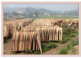
**Figure 12.6.** Veneer air drying.
