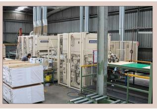
**Figure 9.10.** Automated plywood sanding line.
