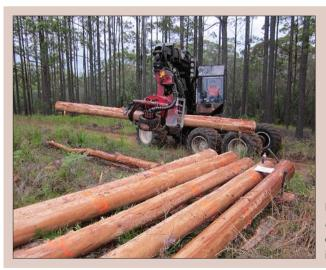
**Figure 3.19.** Mechanised debarking of logs in the forest.
