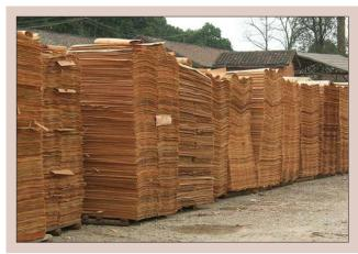
**Figure 12.5.** Veneer sheets after peeling.
