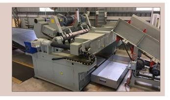
**Figure 4.6.** An example of a spindleless lathe.
