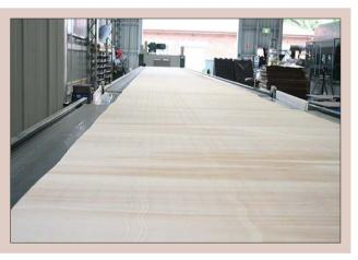
**Figure 5.3.** Veneer ribbon ready for clipping.
