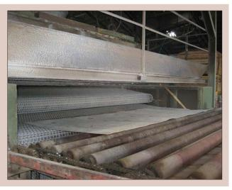
**Figure 5.5.** Jet-box conveyortype veneer dryer.
