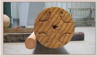
Figure 4.8. A 45 mm peeler core (left) produced from a spindleless veneer lathe, compared with a 130 mm peeler core produced from a standard, commercial spindled lathe.
