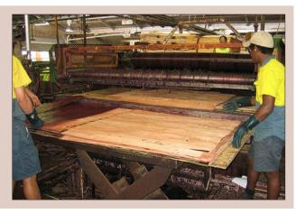
**Figure 9.4.** Glue spreading.
