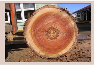
**Figure 3.11.** Significant fungal decay visible on a log end.
