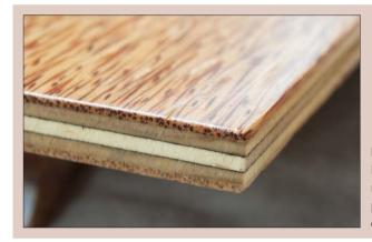
Figure 2.7. Decorative panel made from coconut palm overlaid on plywood.
