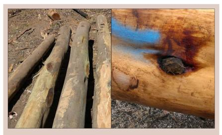
**Figure 3.4.** Knots (old branch stubs) visible on the surface of eucalypt logs (left), and a branch defect that produces an internal knot and hence a veneer defect (right).
