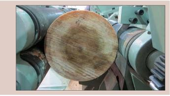
**Figure 4.7.** A log being peeled with a spindleless lathe.
