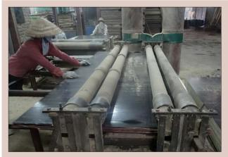
**Figure 9.8.** Panel edge-trimming in Vietnam.
